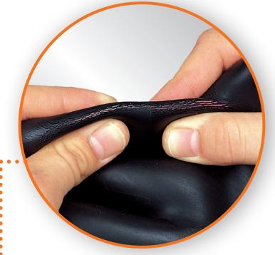
···· CRACKING & CUTTING: Shown above is damage caused by prolonged folding or compressing.
