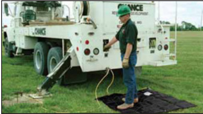
Mechanical Equipment (Vehicles, etc.) Grounding
