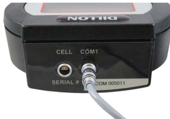
Figure 2.7 External Power Supply Connection (Communicator)
