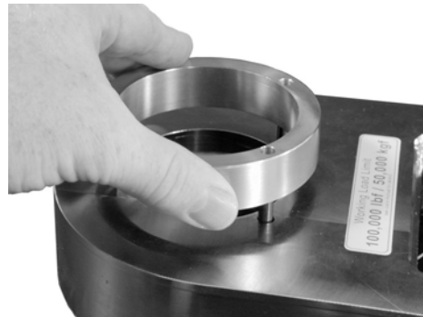
Figure 7.4 Placing Second Spacer on Roll Pins
