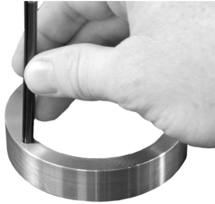
Figure 7.2 Inserting Roll Pin
