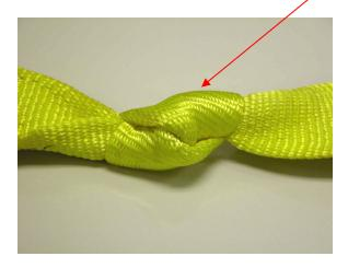
THE DAMAGE: **Broken/Worn Stitching** in the main stitch patterns of web slings has a direct adverse effect on the strength of a sling. The stitch patterns in web slings have been engineered to produce the most strength out of the webbing. If the stitching is not fully intact, the strength of the sling may be affected.
