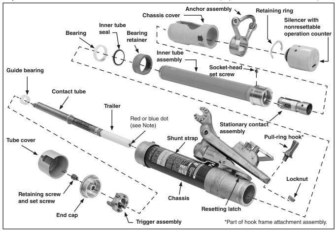
**Note:** Tools with a red dot on the trailer (manufactured before July 2002) can be operated 500 to 1,000 times before inspection and maintenance are required. Tools with a blue
