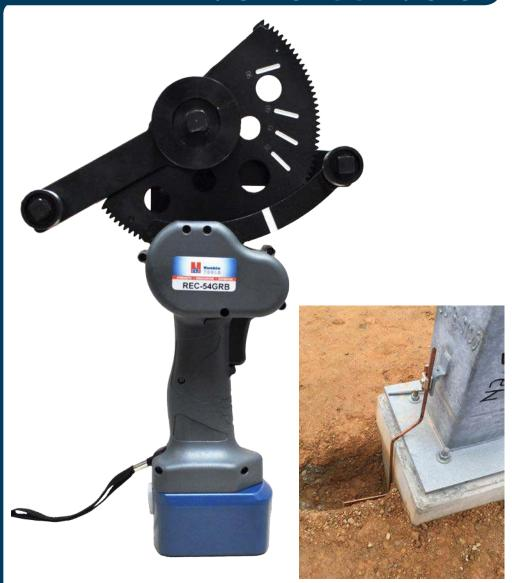
The **REC-54GRB** is a heavy duty copper ground rod bender, primarily used in substations to ground structures and equipment. 4/0 or other size copper used for typical methods of substation grounding can easily be cut and stolen. The REC-54GRB allows you to bend 5/8" ground rods around concrete footings and attach structures directly to the grounding grid while also making it much harder to cut and steal.
